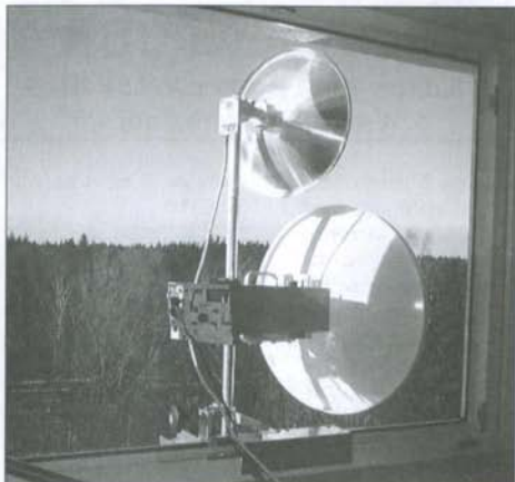
Fig. 1: 24 GHz ATV TRX with 0.48m dish and 0.33m dish above for RX on 10 GHz.
