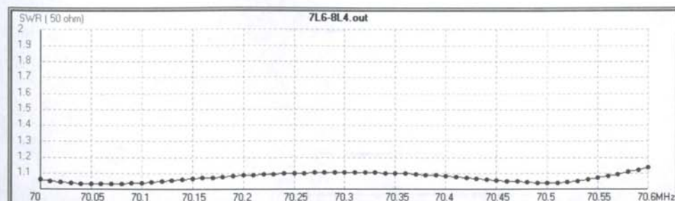
Fig. 12: SWR plot 7 + 8 element yagi for 70 MHz
