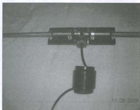
Fig. 18: Driven element with RF choke
