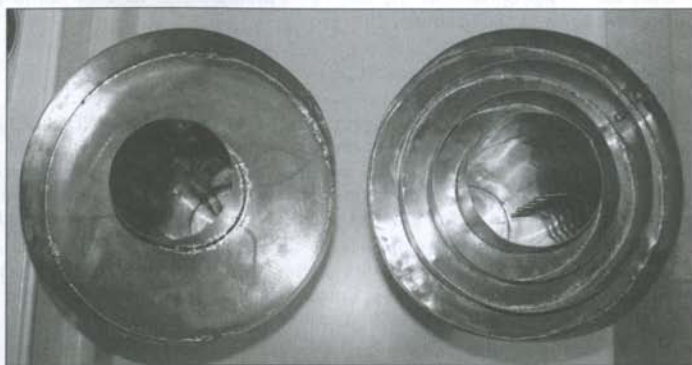
Fig. 19 VE4MA feed with septum polarizer and Chaparral-style feed with screw polarizer
